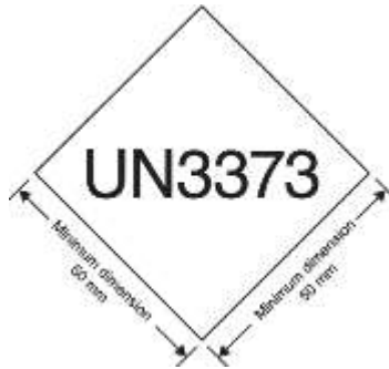
Figure 9: An example of the mark that must be used for Category B Infectious Substances
