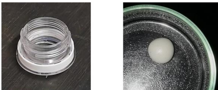
Figure 3. PET bottle neck with tamper-evident ring made of PE and ring converted into a PE pellet.
