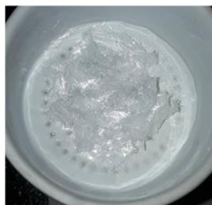
Figure 2. Green PET flakes from a colored plastic bottle and white DMT after depolymerization
