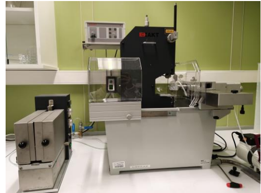
Figure 1. EXAKT equipment used for the processing of mineralized samples and dental materials.
