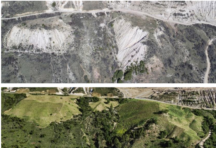
Figure 1. Geomorphic Restoration of the external waste rock dumps of the Santa Engracia mine (Peñalén, Guadalajara, Spain), carried out with the GeoFluv – Natural Regrade method. Left, pre-restoration situation, March of 2020 (photo by Diedro). Right, post-restoration situation, May of 2021 (photo by M.A. Langa)
