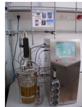
Figure 4. Laboratory-scale MBR (Membrane Bioreactor)
