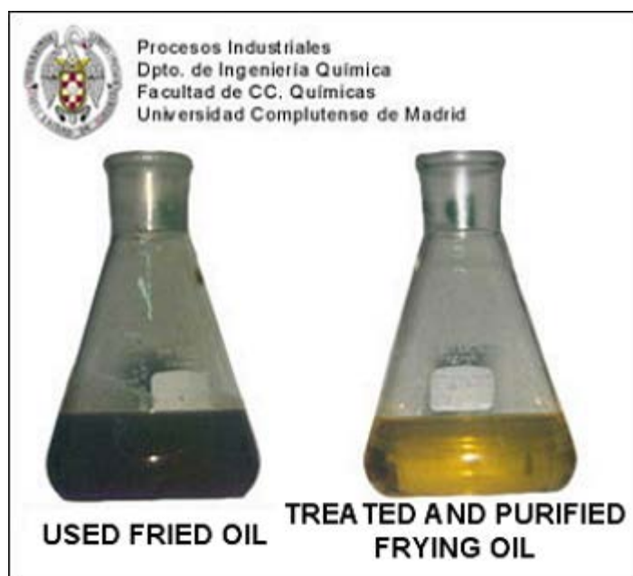
Used frying oil, before and after be subjected to treatment and purification described herein.
