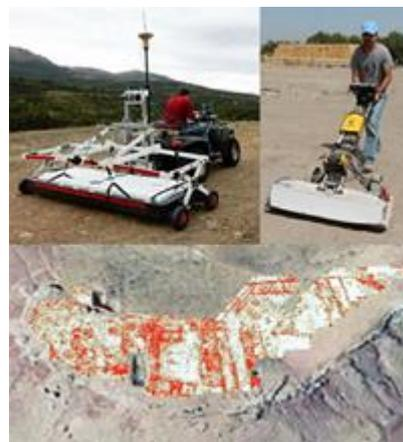
*Multi-channel Ground Penetrating Radar Stream X with antennas of 200 and 600 MHz. Detection of underground structures in El Castillón (Ciudad Real).*
