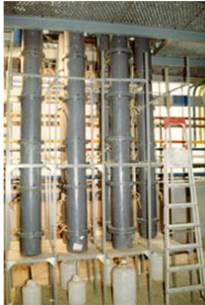
Figure 2. Bioleaching columns: treatment of uranium ores at semi-pilot scale.
