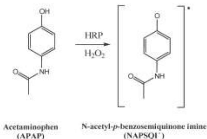
Scheme 8. Production of NAPSQI• from APAP via HRP-Catalyzed Oxidation in the Presence of H 2 O 2 .
