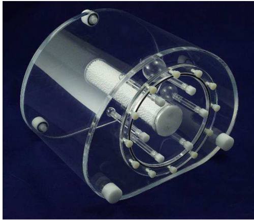
(a) NEMA IEC PET Body Phantom (NU2 2018)™ [19]
