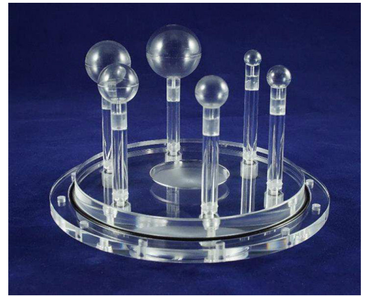
(b) NEMA IEC PET Body / CT Lid with Hollow Spheres [19]
