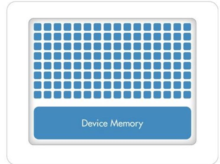
“A CPU consists of a few cores optimized for sequential serial processing while a GPU has a massively parallel architecture consisting of thousands of smaller, more efficient cores designed for handling multiple tasks simultaneously.”
