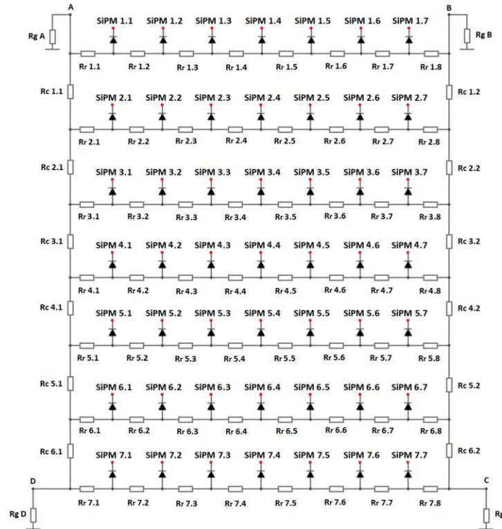
Multiplexing the SiPMs of the array to reduce the 8x8 outputs to 4, taking the signals from each corner
