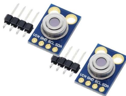
Figura 15. Sensores TECNOIOT MLX90614ESF. Fuente: https://www.amazon.es/Hailege-MLX90614-Non-Contact-Temperature-Raspberry/dp/B07YKNQQ7P
