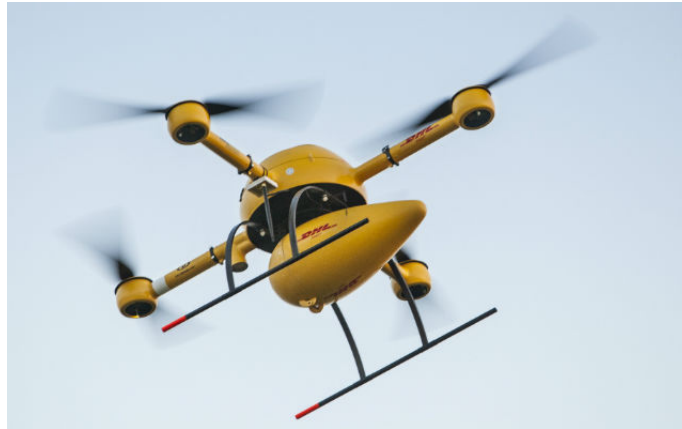
Figure 5.2: Example of quadcopter with its payload covered with a nacelle. The direction of flight must be aligned with it.
