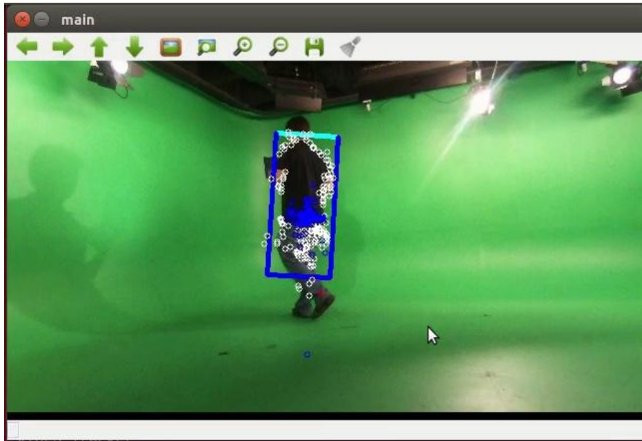
Figura 47. Tracking indoor controlado detector FAST
