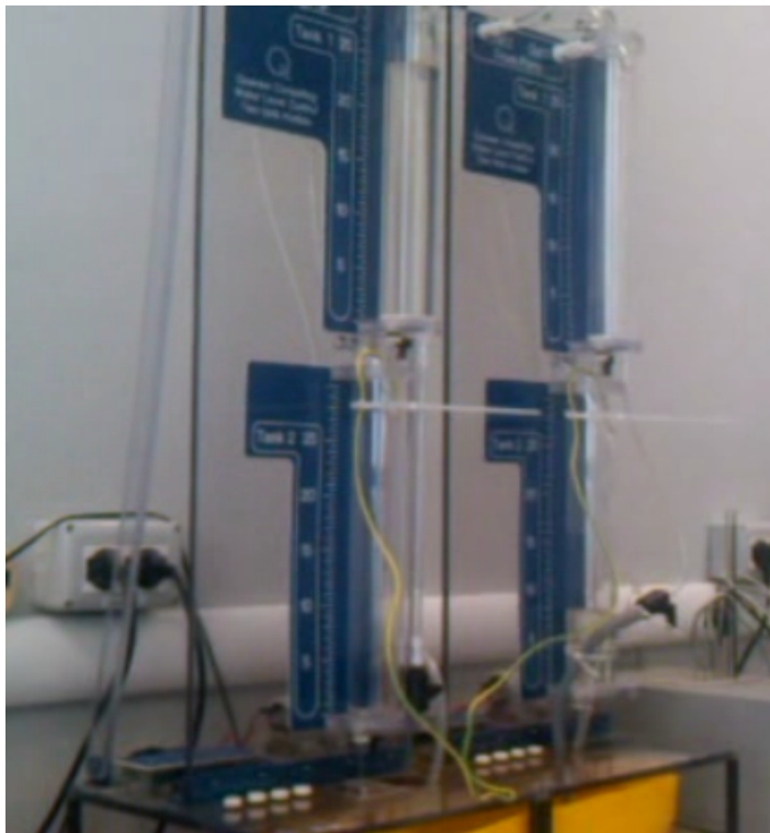
Figure 3.1: Two-Tank System from Quanser.
