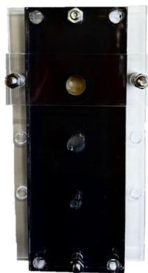
Figure 2. Black-coated PMMA sample holder with a 1 cm diameter cavity containing a shredded wool yarn button.
