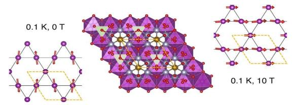
Structure of  $FeMn_3Ge_2Sn_7O_{16}$  (Fe = gold,  $MnO_6 = purple$ , Sn = grey,  $GeO_4 = green$ , O = red) with its zero-field and in-field magnetic structures.
