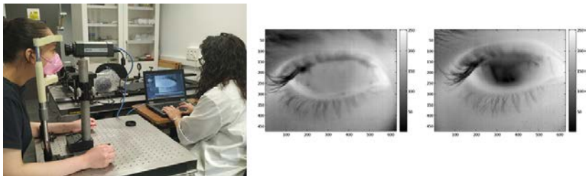
Figure 1: From left to right: experimental set up, thermal image baseline and with contact lens.
