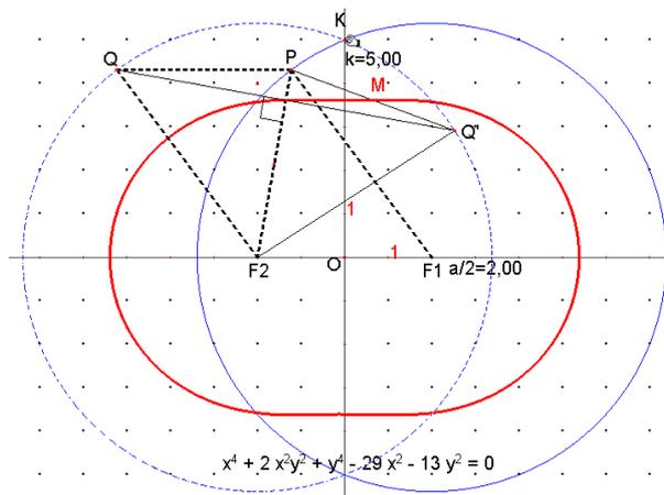
Fig. 4.3: Embedded coupler curve with its equation and variation of  $k$ -values
