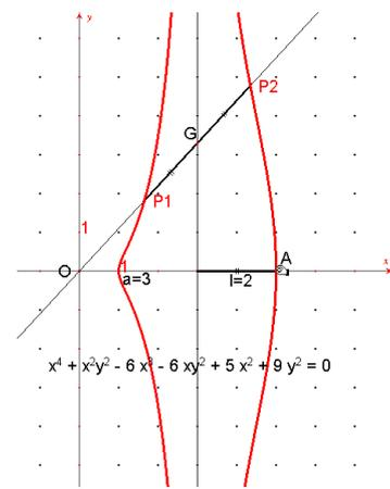
Fig.2.21: Nicomedes Conchoid's construction and equation
