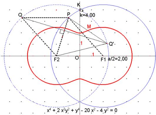
Fig. 4.2: Embedded coupler curve with its equation and variation of  $k$ -values
