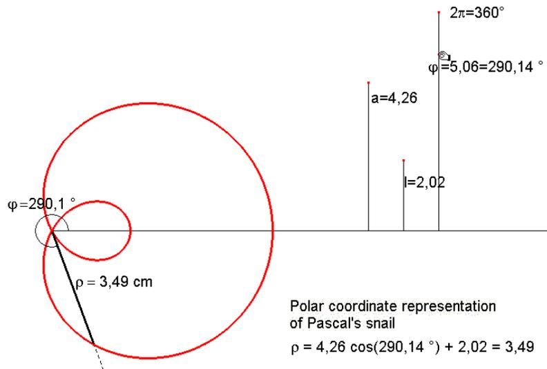
Fig. 2.18: Polar coordinate representation of Pascal's limaçon
