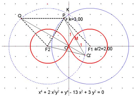
Fig. 4.1: Embedded coupler curve with its equation and variation of  $k$ -values
