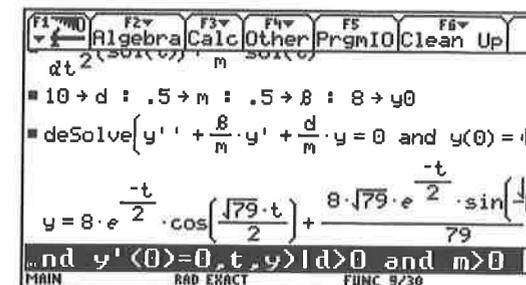
Figure 4: Solution with discrete parameters,  $d = 10$ ,  $m = 0.5$ ,  $\beta = 0.5$  and  $y_0 = 8$ .
