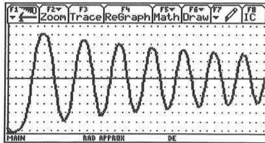
Figure 13: Simulation of the angular displacement of a physical pendulum by means of the ODE (7)
