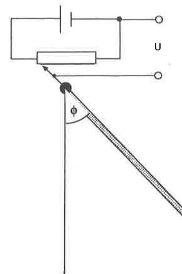
Figure 6: Sketch of the physical pendulum, the angle is measured by the voltage at the potentiometer.
