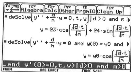
Figure 2: Particular solution for an undamped oscillation.
