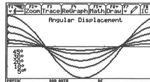
Figure 11: Oscillations with initial displacements between  $45^\circ$  and  $5^\circ$ .
