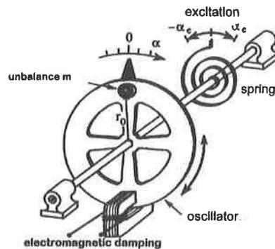
Figure 14: Sketch of a driven rotational pendulum with an unbalance
