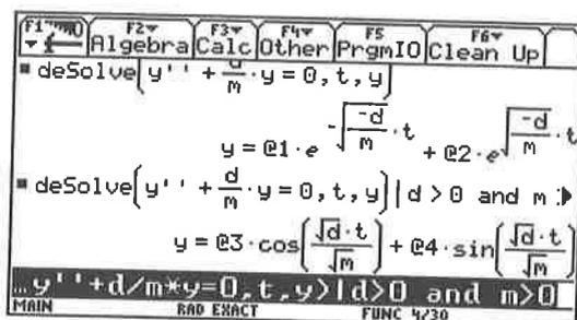
Figure 1: General solution for an undamped oscillation.
