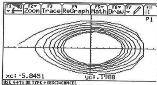
Figure 9: Phase diagram of the physical pendulum
