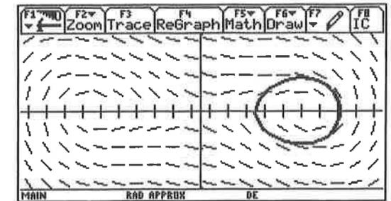
Figure 15: Phase portrait of a quasi harmonic oscillations of a rotational pendulum with an unbalance
