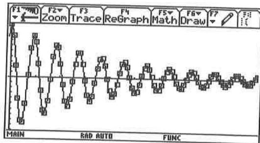
Figure 5: Comparison of the exact(x-y line) and the numerical(squares) solution of equation (3)
