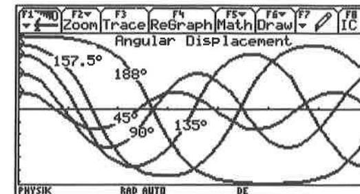
Figure 10: Oscillations with initial displacements between  $179^\circ$  and  $90^\circ$ .
