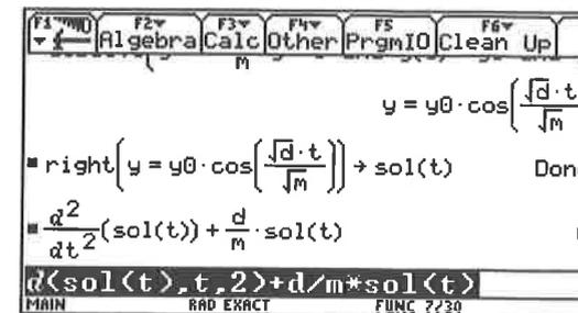
Figure 3: Verification that  $sol(t)$  is a solution of equation (1).
