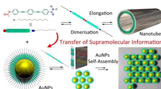
Figure 1: Scheme of the hierarchical self-assembly of AuNPs and OPE molecules.
