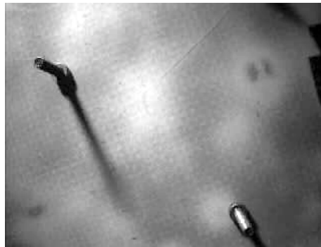
Fig. 8. (1.07 MB Movie). When moving the grating it is easier to distinguish real surface deviations from external inclusions (dirt and air bubbles) which have different behaviors. The tissue texture appreciated in the picture is due to the structural nature of the composite panel. There are two screws on the plastic grating as a reference.
