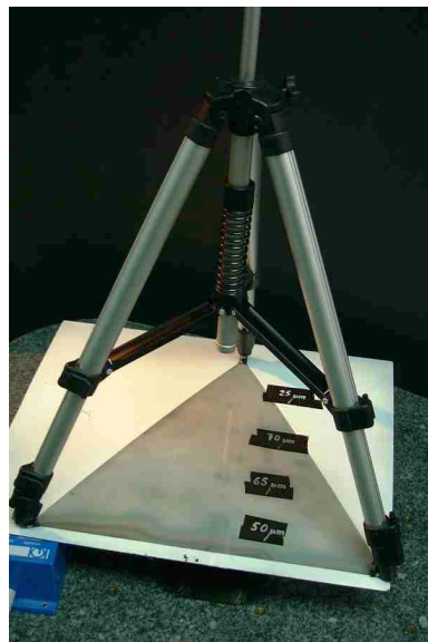
Fig. 5: Tripod solution for the adaptation of flexible gratings to curved surfaces. The grating is stretched between three contacting points. Tensile load is provided by a spring. The uniform gray appearance of the grating is a signal of good adaptation to the curved surface. Local profile deviations produce a stain like appearance. The source is a commercial 50 W halogen lamp with a dichroic reflector and a rectangle narrow aperture aligned parallel to the grating.
