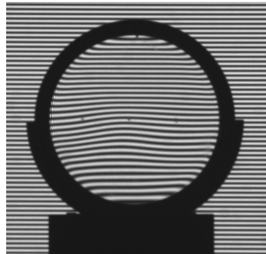
Fig. 2 Fringe pattern obtained with the progressive lens placed at 10.0 mm from the screen.
