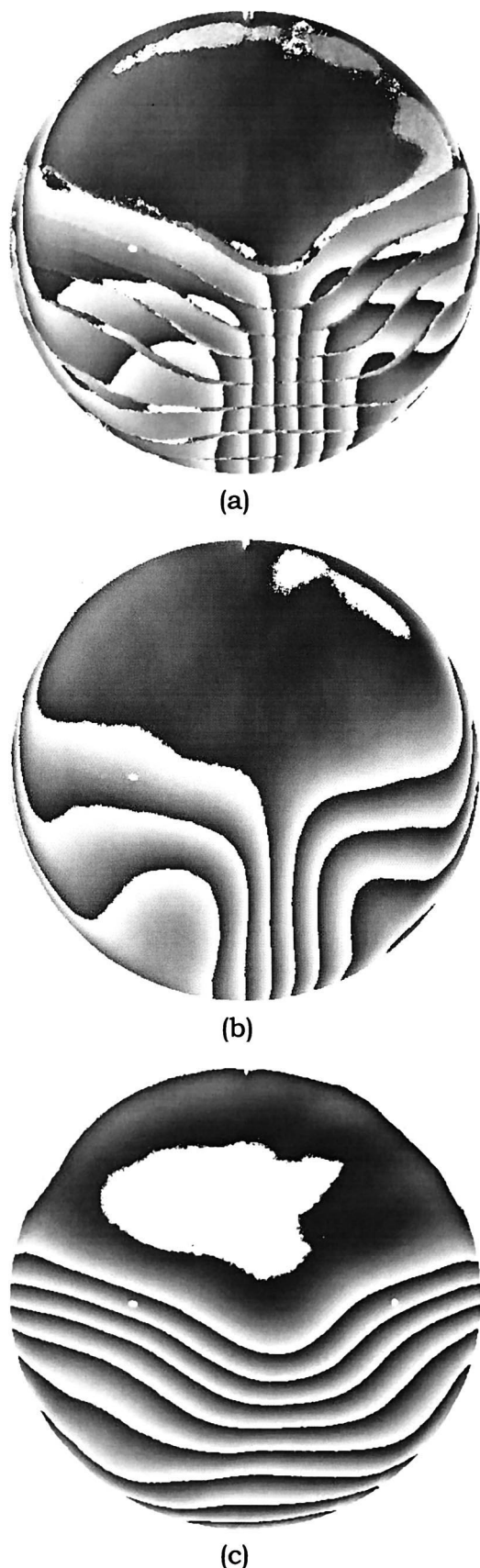
Fig. 5. (a) Phase map associated with the x -deflection component obtained with Eq. (7). The low-modulation areas corrupt the information. (b) Phase map associated with the x -deflection component obtained with Eq. (10). The low-modulation areas were
