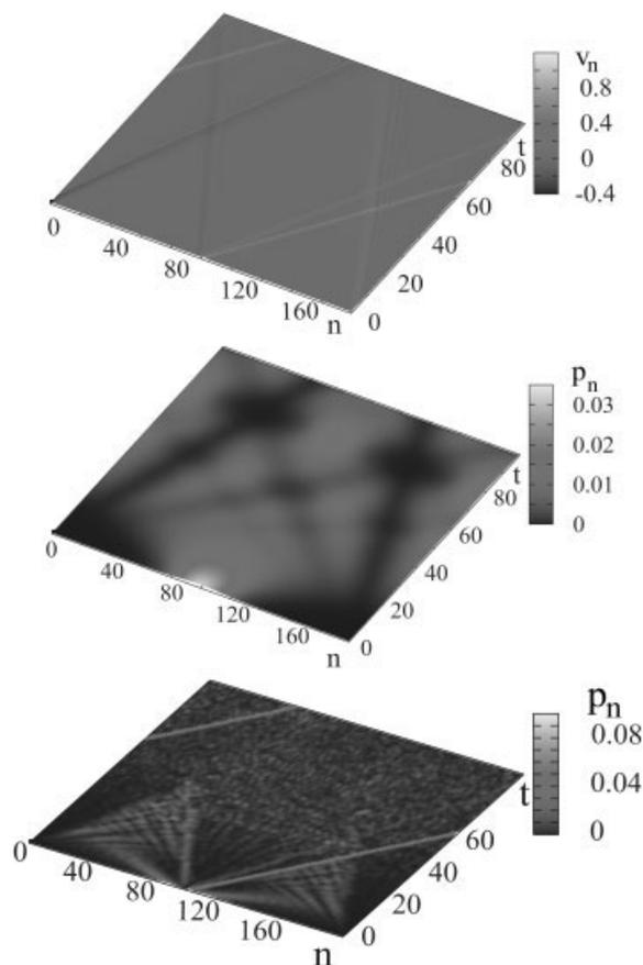
**FIGURE 4.** Toda–Morse lattice. Results of numerical integration of Eqs. (12) and (13). Upper figure:  $\alpha = 0$ , soliton alone; center figure:  $\alpha = 0$ , electron alone; lower figure:  $\alpha = 1,75$ , solectron (electron dynamically bound to the soliton). The gray scales (velocity and probability density) are in arbitrary units, just for illustration.
