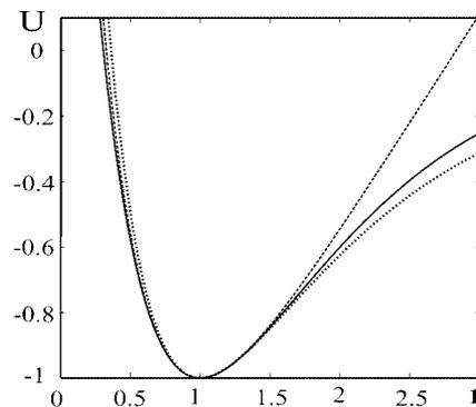
**FIGURE 1.** The available knowledge about depth, frequency, and stiffness of the interaction of atoms may be fitted by different potentials. Here, Toda (upper curve), Morse (middle curve), and  $(r^{-12}, r^{-6})$  Lennard-Jones potentials suitably scaled around the minimum to have identical second and third derivatives. Relevant in our context is the repulsive part.
