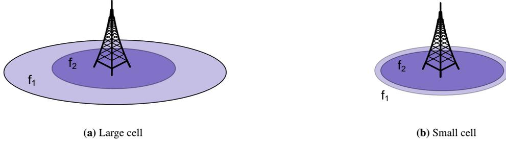
**Figure 4:** Illustration of the propagation differences between frequencies in multicarrier BS in large and small cells.
