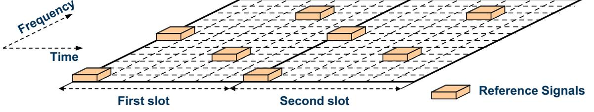
**Figure 3:** Illustration of the Cell-specific Reference Signals in an LTE network. Source: based on Dahlman et al. (2014)
