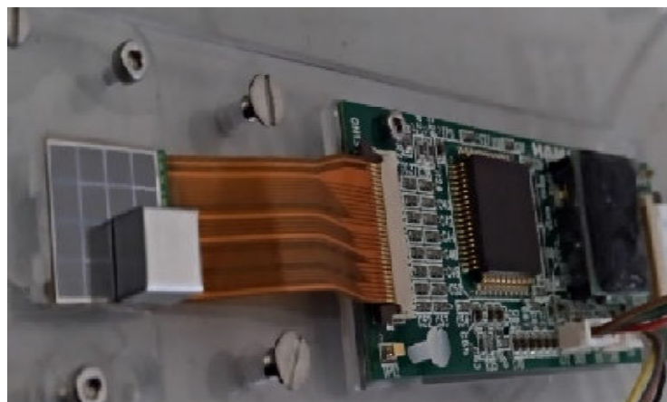
Setup for gamma-ray spectroscopy with scintillator, J. Rosado et al.
