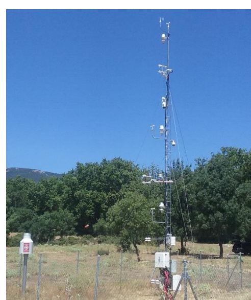
Figure 3. Picture of the 10-m meteorological fixed tower at La Herrería Forest during Summer 2017. Wind speed and temperature are measured at 3, 6 and 10 m with cup anemometers and aspirated thermometers respectively, and wind direction at 10 m with a wind vane. CO 2 and water-vapour concentration and turbulent fluxes are measured at 4 and 8 m with IRGASON devices. Besides, precipitation and soil-humidity measurements are also carried out. La Herrería is part of the Guadarrama Monitoring Network ( GuMNet ; www.ucm.es/gumnet/ ).
