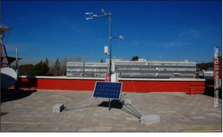
Figure 13. Station scheme on the left, a picture on the right .The EG901- Portátil is a portable automatic weather station design to monitor turbulent processes responsible for soil respiration and gas exchange, such as turbulence CO2 and H2O vapor fluxes, take place in this range.
