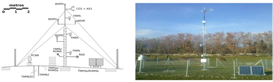
Figure 12. Station scheme on the left, a picture on the right. EG010- La Herrería automatic weather station is located in the municipality of El Escorial at 920 m.a.s.l. Atmospheric instrumentation have been design to study boundary layer evolution and CO2 fluxes.
