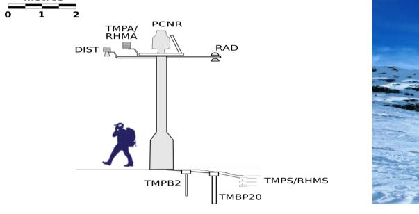
Figure 11. EG006-Hoyas automatic weather station is located in the circue valley of Peñalara at 2.019 m.a.s.l. Abounding in tall grass and wetlands, the design of the station aims to minimal impact without perimeter security fence. A single mast houses all the atmospheric instrumentation. Since it is located in an area of high accumulation of snow during the winter season, the mast is configured to be over the snow cover and high visible to avoid ski activities.
