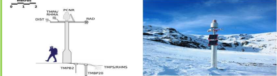
Figure 11. EG006-Hoyas automatic weather station is located in the cirque valley of Peñalara at 2,019 m.a.s.l. Abounding in tall grass and wetlands, the design of the station aims to minimal impact without perimeter security fence. A single mast houses all the atmospheric instrumentation. Since it is located in an area of high accumulation of snow during the winter season, the mast is configured to be over the snow cover and high visible to avoid ski activities.
