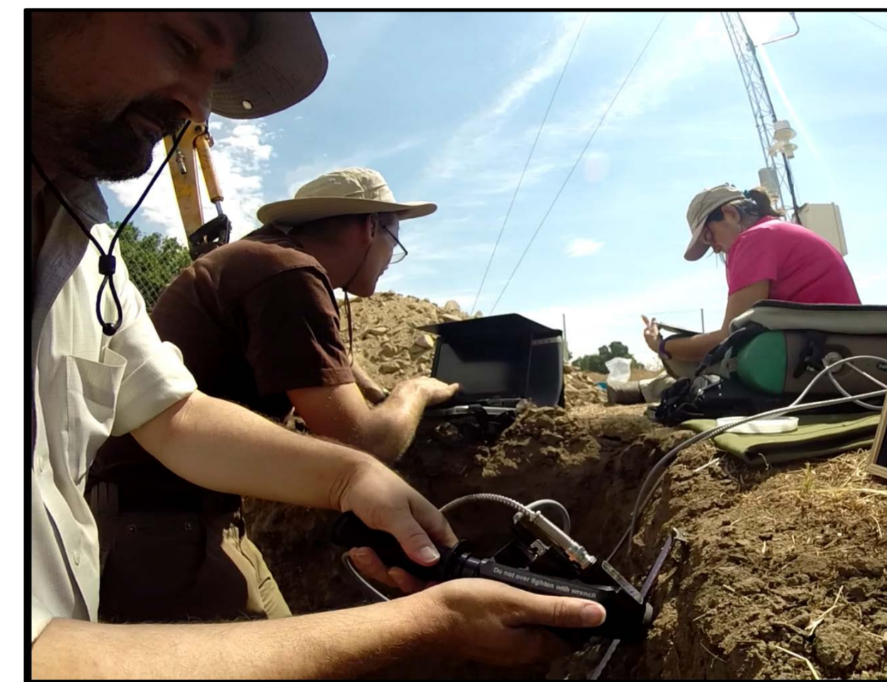
Fig. 4. The use of reflectant spectroscopy allows to characterize the chemical composition, as well as the water content, of the different layers of the subsurface. Once the spectroscopy analysis is done, a set of samples are taken in order to realize future analysis in the laboratory. And finally before covering the trench, the temperature and humidity sensors are placed at different depths.
