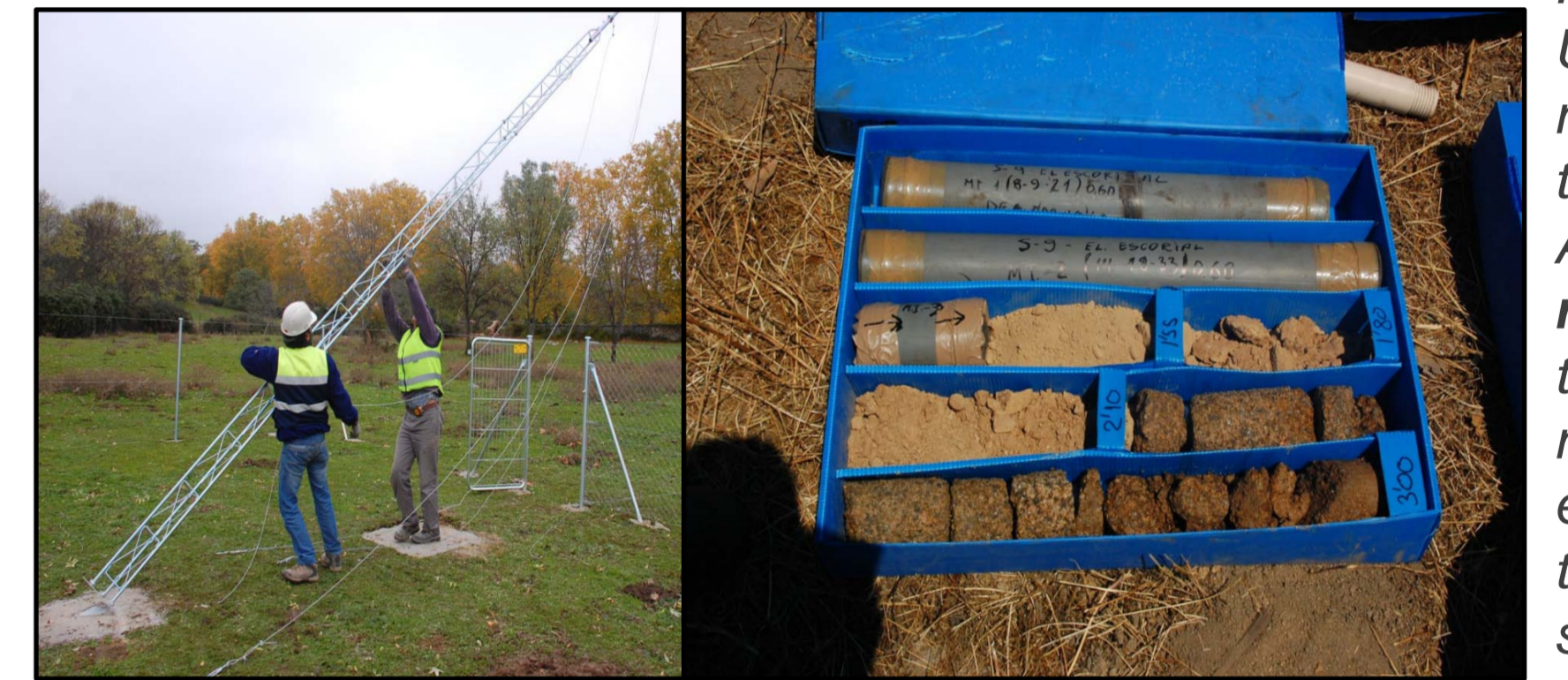
Fig. 4. The use of reflectant spectroscopy allows to characterize the chemical composition, as well as the water content, of the different layers of the subsurface. Once the spectroscopy analysis is done, a set of samples are taken in order to realize future analysis in the laboratory. And finally before covering the trench, the temperature and humidity sensors are placed at different depths.
