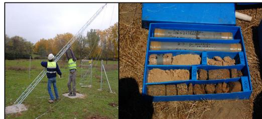
Fig. 3. (a) Left: Uprising of the meteorological tower. (b) Right: A set of core rocks. Note that the first 1.5 meters are encased in PVC to preserve the soil structure and composition.
