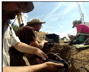
Fig. 4. The use of reflectant spectroscopy allows to characterize the chemical composition, as well as the water content, of the different layers of the subsurface. Once the spectroscopy analysis is done, a set of samples are taken in order to realize future analysis in the laboratory. And finally before covering the trench, the temperature and humidity sensors are placed at different depths.
