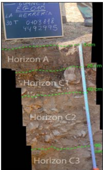
Figure 1. Detail of the different soil horizons characterized in the EG010-La Herreria trench.
