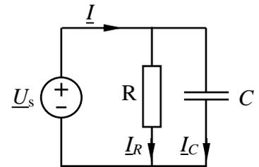
DATOS:  $u_s = 50\sqrt{2} \cos 1000t \text{ V}$ ,  $R = 25 \Omega$ ,  $C = 0,02 \text{ mF}$ .
