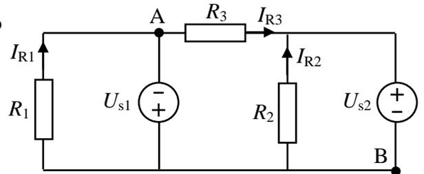
DATOS:  $R_1 = 2 \Omega$ ,  $R_2 = 40 \Omega$ ,  $R_3 = 5 \Omega$ ,  $U_{s1} = 10 \text{ V}$ ,  $U_{s2} = 20 \text{ V}$ .
