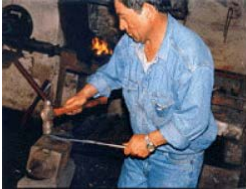
Forging process of Damascus steel and example of finished knife.
