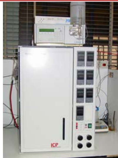
Continuous reactor under subcritical conditions with downward flow (TBR).
