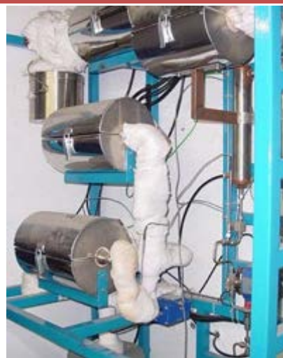
Continuous reactor working in supercritical conditions.
