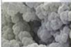
Carbon granules (here magnified around 4,000 times) from a filter trap the contaminants like a magnet as the water flows through.
