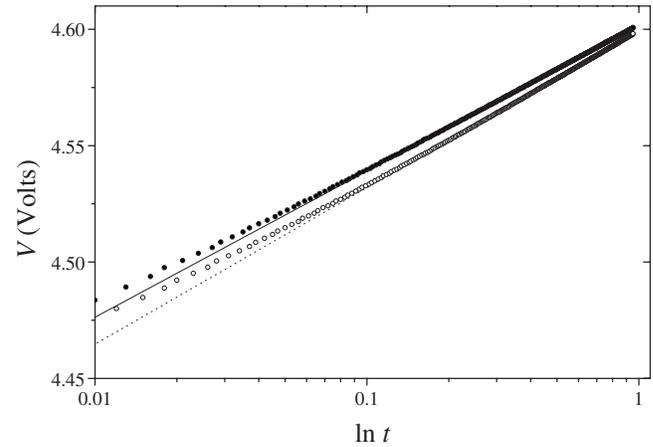
FIG. 1. Typical individual heating curves: voltage drop in the wire,  $V$ , as a function of time  $t$ . Open symbols are for pure EG and filled symbols are for the nanofluid prepared by dispersing silica nanoparticles in glycol at 4.8% (w/w). In both cases the initial temperature was 60 °C and  $I=320$  mA. Straight lines represent fittings to Eq. (1) of the points measured after  $\approx 213$  ms.
