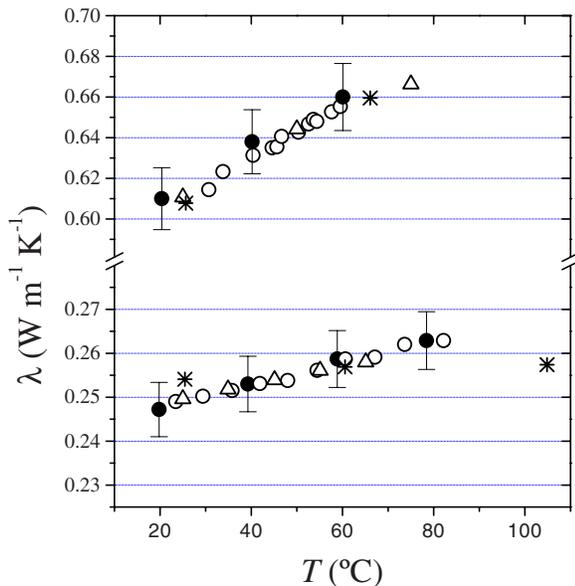
FIG. 2. (Color online) Comparison of the thermal conductivity values obtained in this research (filled circles) with several literature values. For water (top panel) triangles are from the ASTM-D2717 standard, empty circles are from Assael *et al.* (Ref. 30), and asterisks are from Bohne *et al.* (Ref. 31). For EG (bottom panel) triangles are from Khayet and Ortiz de Zárate (Ref. 23), empty circles are from Assael *et al.* (Ref. 30), and asterisks are from DiGiulio and Teja (Ref. 32).
