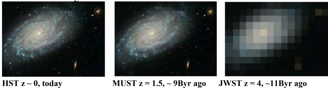
Figure 2: Three images of the same galaxy, under varying assumptions. The MUST image assumes a galaxy diameter of 1'' at 0.01'' resolution; the JWST image assumes a galaxy diameter of 0.6'' at 0.068'' resolution ( 0.068'' = \lambda/D for 2\mu\text{m}/6\text{m} ). (Galaxy diameters from Ferguson et al, 2004.)
