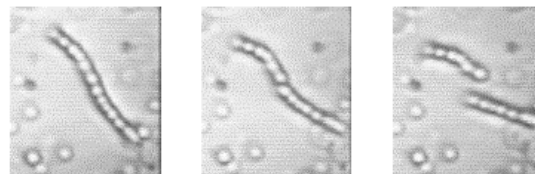
Figure 3. Detail of the S shape of a chain induced on the same suspensions when a magnetic field of amplitude H=1.55 kA/m rotates counter clockwise with f = 0.01 Hz. Field of View: 14.4 \times 14.2 \mu\text{m}
