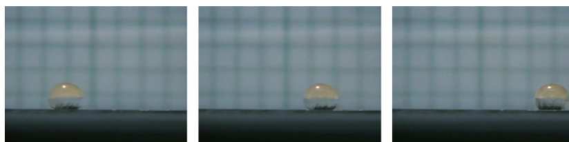
Fig. 2. Still frames from a video showing the movement of a 20 \mu l water drop containing 2% carbonyl iron particles. The drop moves from left to right by the action of a permanent magnet that is manually displaced below the surface and reaches a maximum speed of about 2 cm/s.
