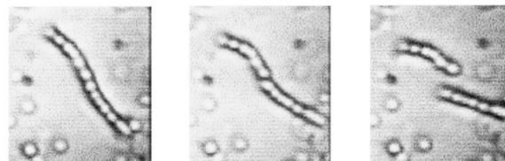
FIG. 6. Detail of the S shape developed by a critical chain in a counterclockwise rotating field of amplitude 1.55 kA/m (19.5 Oe) and frequency 0.01 Hz. These chains formed in an aqueous dispersion of 1.24-mm-diam soft magnetic particles at volume fraction 0.001.
