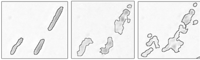
Fig. 9. Example of chains disaggregating for different times in the experiment \lambda = 77 and \phi_{2D} = 0.071 . The contour around the chains is the border of the clusters detected by means of the image analysis, while the grey color is the original captured image. Left: t = 0 s (when field is off), middle: t = 20 s, and right: t = 40 s.
