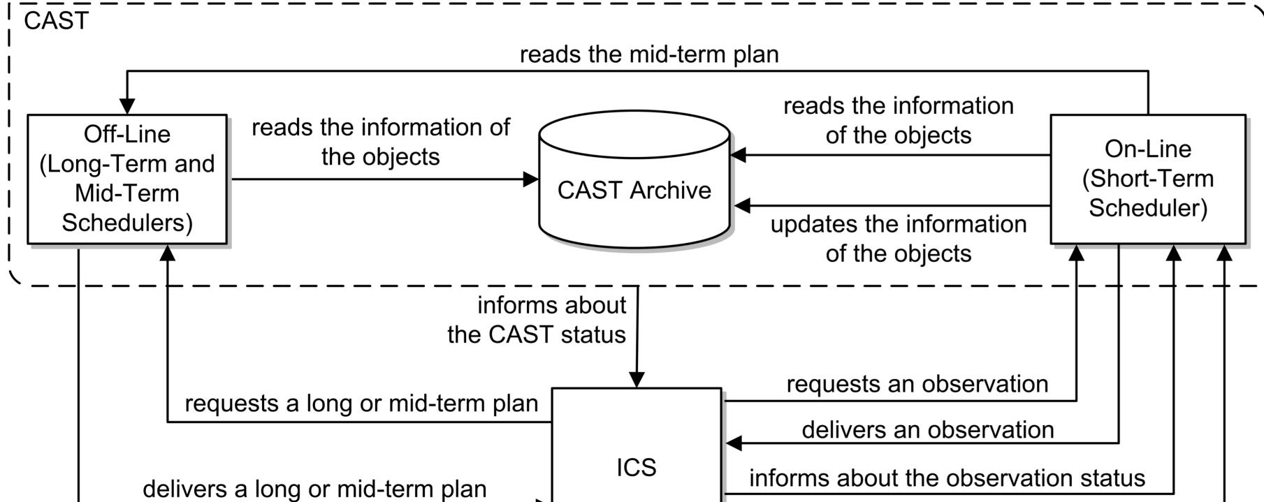
The communications between the ICS and CAST are done by means of the Internet Communication Engine (ICE) protocol:
