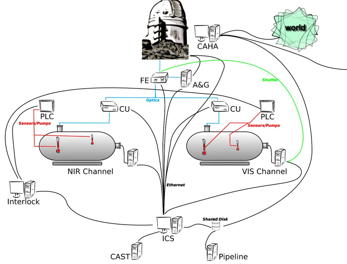
The Instrument Control System (ICS) is the central software application in
