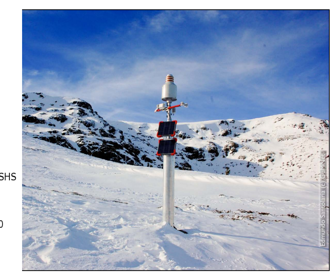
Fig 10. EG006-Hoyas automatic weather station is located in the cirque valley of Peñalara at 2,019 m.a.s.l. Abounding in tall grass and wetlands the designe of the station amis to minimal impact without perimeter security fence. A single mast houses all atmopheric instrumentation. Since it is located in an area of high accumulation of snow during the winter season, the mast is configured to be over the snow cover and high visible to avoid ski activities.
