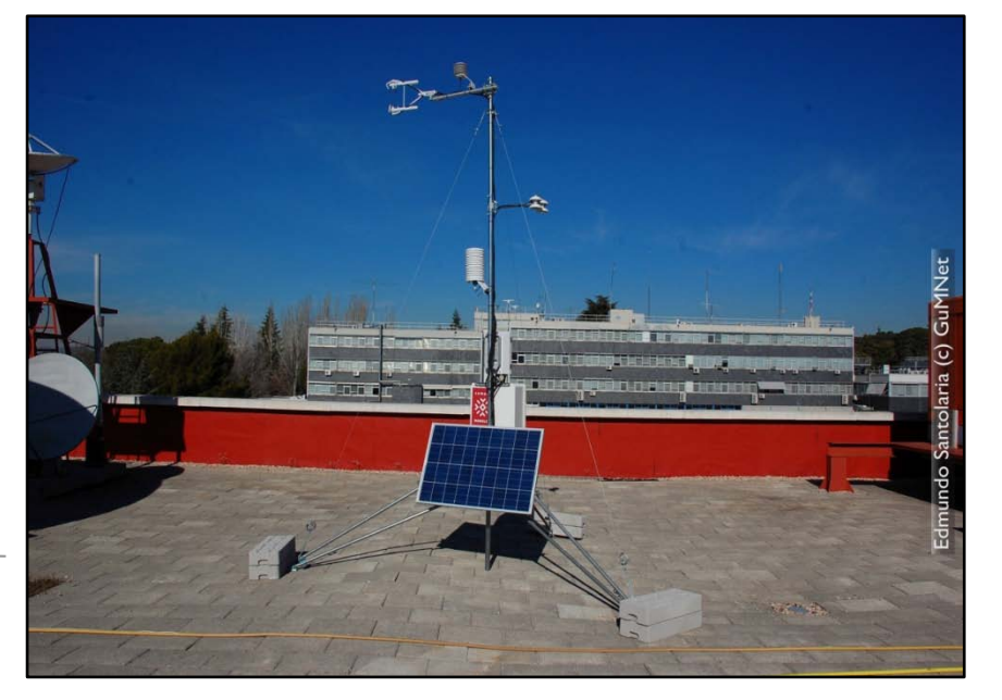
Fig 8. left scheme, right picture) The EG009- Portatil is a portable automatic weather station design to monitor turbulent processes responsible for soil respiration and gas exchange, such as turbulence CO 2 and H 2 O vapor fluxes, take place in this range.
