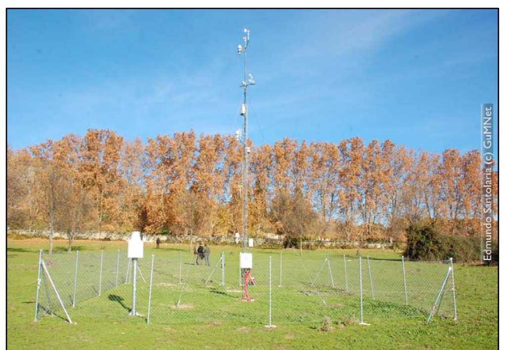
Fig 7. (left scheme, right picture) EG010- La Herreria automatic weather station is located in the municipality of El Escorial at 920 m.a.s.l. Atmospheric instrumentation have been design to study boundary layer evolution and CO 2 fluxes.
