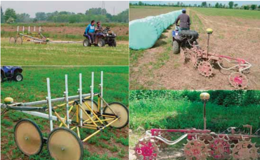
Figure 2. Geophysical instruments used during the survey. Left: the Automatic Magnetic Profiler (AMP© Geocarta), capable of recording up to 20ha each day. Right: the Automatic Resistivity Profiler (ARP© Geocarta), capable of recording up to 4ha each day. To increase productivity within the project two ARP instruments were often used simultaneously.
