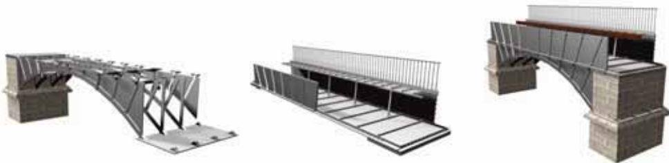
Figure 10. Still images from the Pontcysyllte video presentation. The images show successive stages in the mounting of the cast-iron canal trough on the aqueduct's supporting piers [6]
