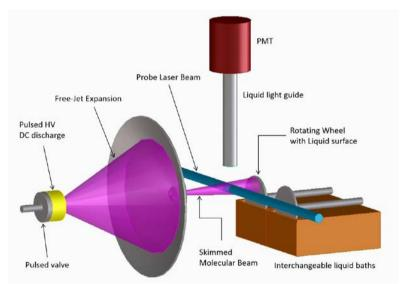
Figure: A schematic of the pulsed OD molecular beam / liquid-surface scattering apparatus. **Acknowledgments:** This work has the support of Heriot-Watt University through the provision of a James-Watt Scholarship for R.H.B.
