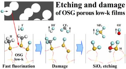
Fig. 1: Schematic stages of OSG films etching and damage by fluorine atoms. **Acknowledgments:** This work is supported by Russian Scientific Fund (16-12-10361).
