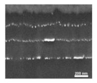
Figure 1.: SEM micrograph of the transversal section of a multilayer structure (Ag/SiO<sub>2</sub>/Ag/SiO<sub>2</sub>/Ag/SiO<sub>2</sub>) deposited on a silica substrate.
