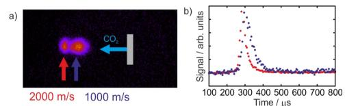
Figure 1. a) Ion image showing two different velocity components for CO<sub>2</sub> formed on the Pt(111) surface. b) The time dependence of the signal in the different channels measured by the delay between the molecular beam pulse and the ionization laser.
