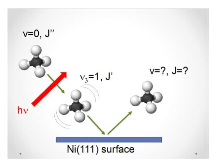
Figure 1: Schematic of the state-to-state methane scattering experiment
