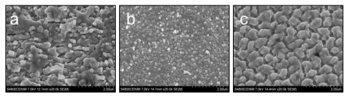
Fig 1. SEM micrographs of titanium alloys irradiated with a) 800, b) 400 and c) 266 nm.
