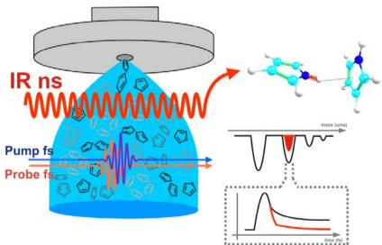
Figure: Schematic representation of the IR tagged time resolved ionization method. Acknowledgments: This work has the support of Spanish MINECO and the Basque Government. The experiments were carried out at SGIker Laser facility (UPV/EHU).
