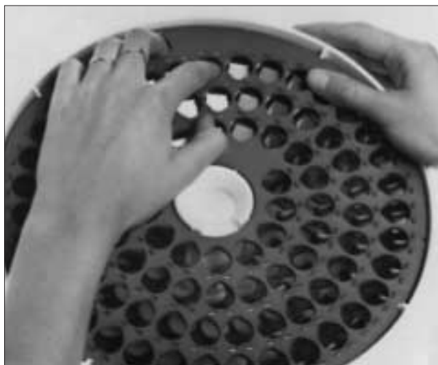
Fig. 10. Snapping the tube holder into place.
